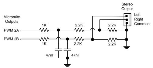
This is suitable for general use, however more sophisticated designs can be implemented if required to improve the frequency response and reject more of the carrier frequency. This circuit is also suitable for generating a DC output signal using the PWM commands although in that case both the 47 nF capacitors should be increased to  $4.7 \,\mu\text{F}$ .
