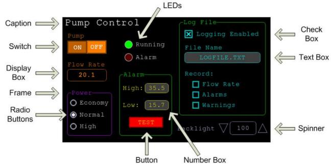
Each control has a reference number called '#ref' in the description of the control. By default this can be any number between 1 and 100 and the upper limit can be changed with the OPTION CONTROL command. The reference number is used to identify a control. For example, a check box can be created thus:
