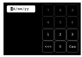
The value of the control can be pulled apart using the string functions or, in some cases, the string can be used directly. For example, if using the above format box to get a date from the user the Micromite's internal clock could then be directly set as follows:
