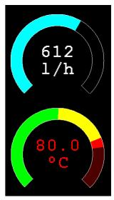
When colours and thresholds are specified the background of the gauge will be drawn with a dull version of the gauge colour at that level ("ghost colouring") so that the user can appreciate how close to the various thresholds the actual value is. Also the digital value displayed in the centre will also change to the colour specified by the current value.
