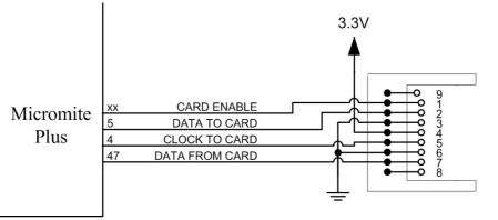
Care must be taken with display panels that share the SPI port between a number of devices (SD card, touch, etc). In this case all the Chip Select signals must configured in MMBasic or alternatively disabled by a permanent connection to 3.3V. If this is not done any floating Chip Select signal lines will cause the wrong controller to respond to commands on the SPI bus.
